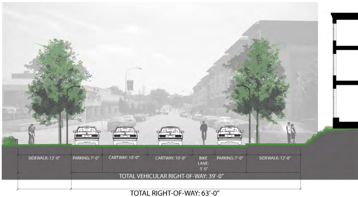
Chestnut Street Top: Existing street section, Bottom: Proposed lane removal, bike lane addition and landscaped buffers.
