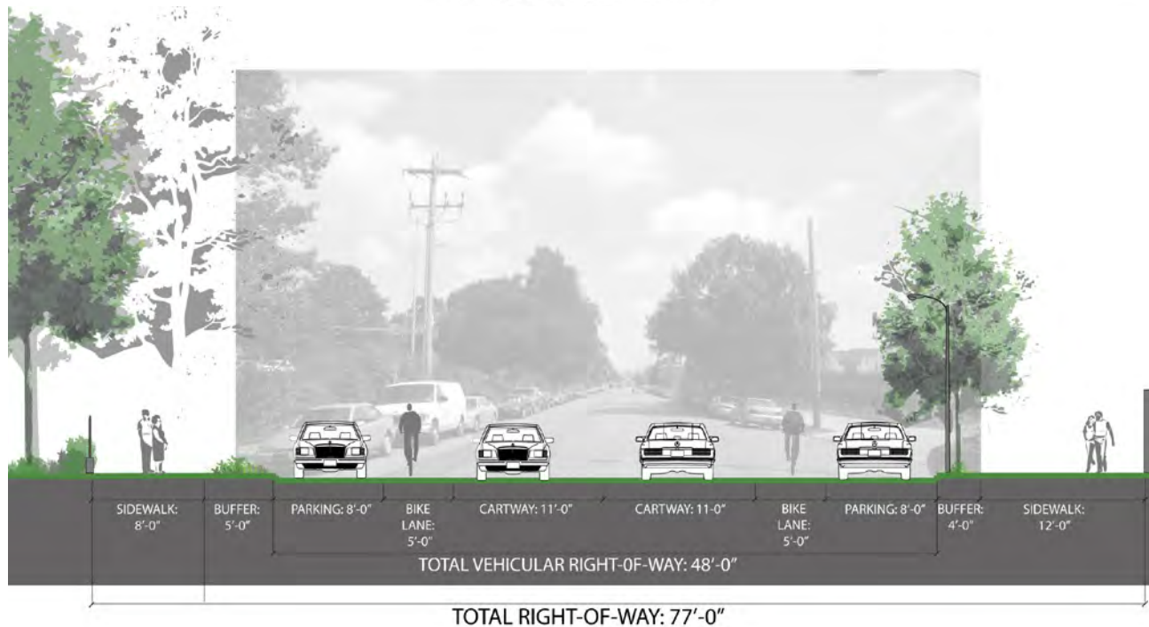
North 46th Street Top: Existing street section Bottom: Proposed travel lane reductions and bike lane additions
