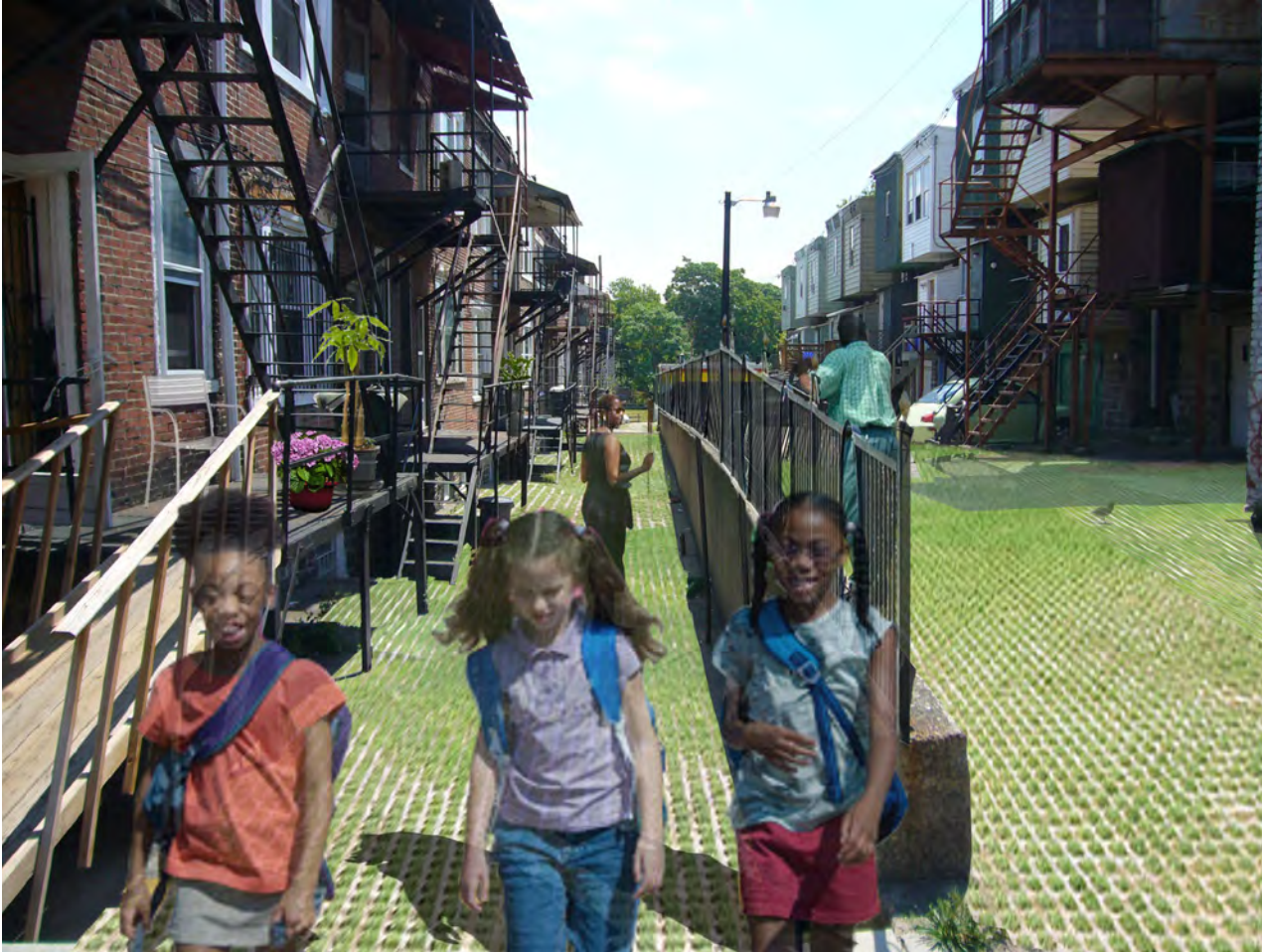
Alleyway treatment Top: Existing paving Left: Proposed permeable paving
