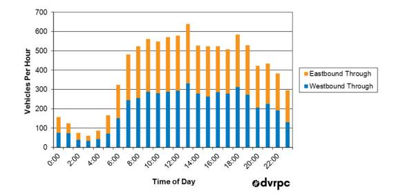
Figure 5: 24-hour Profile of Vehicular Traffic on Main Street by Direction
