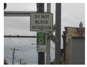
Above: A cross buck sign is obscured by a "Trolley Stop" sign and "Do Not Block Intersection" sign on the eastbound approach to the grade crossing on Main Street. (Source DVRPC)
