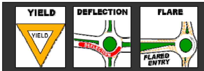
Figure 1 – 3 Basic Design Features of a Roundabout
